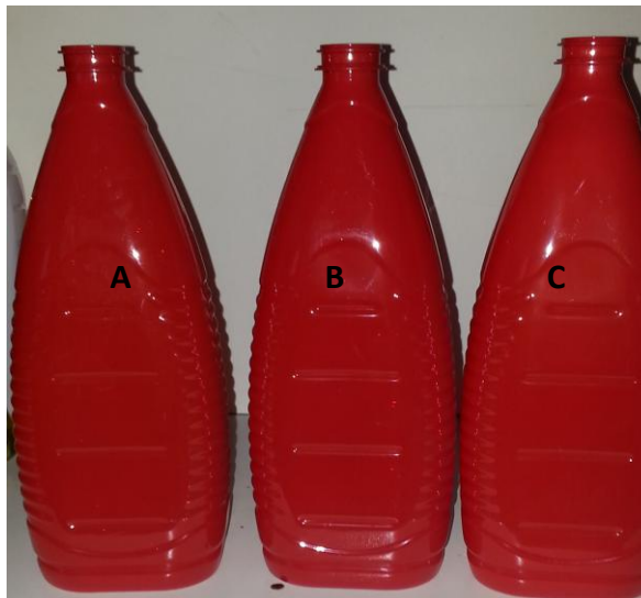
Figure 4. Red 1 liter bottle for seeds olis (OLITA design). A) 31g 100% V-PET bottle; B) 31g 50% R-PET/V-PET bottle; C) 31g 100% R-PET bottles.
