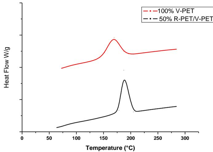
**Figure 5.** Cooling thermograms of 100% V-PET and 50% R-PET/V-PET preforms
