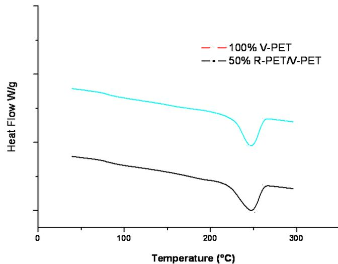
**Figure 6.** Second Heating thermograms of 100% V-PET and 50% R-PET/V-PET preforms
