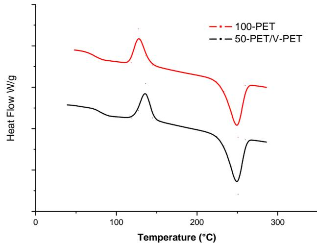
**Figure 4.** First Heating thermograms of 100% V-PET and 50% R-PET/V-PET preforms
