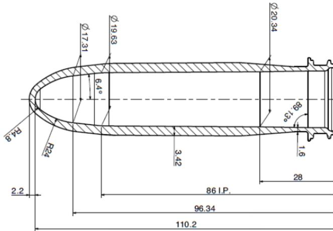
**Figure 3.** Technical drawing of 31g preform, designed by SIAPI for RE-PACKEDOILS Project.
