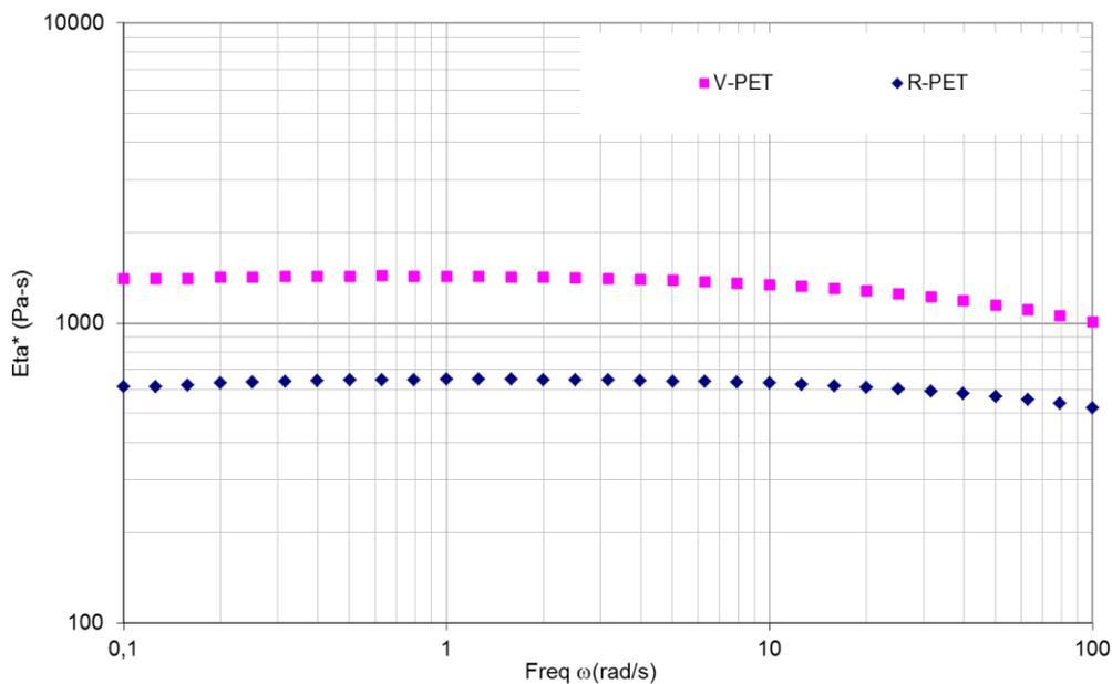
**Figure 2.** Complex viscosity curve in function of frequency for V-PET and R-PET used for preform production evaluated at 280°C and 20% strain.
