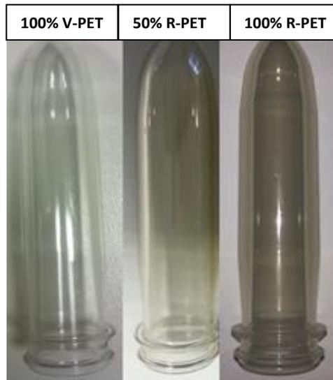
**Figure 1:** 31g PET preforms clear produced during the RE-PACK EDOILS Project.
