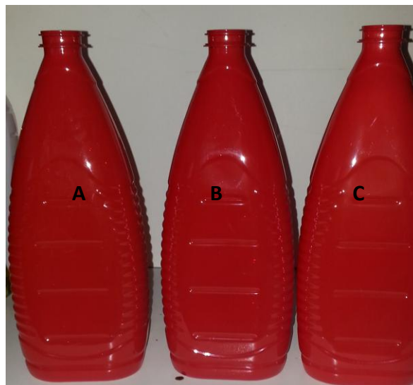
Figure 4. Red 1 liter bottle for seeds oils (OLITA design). A) 31g 100% V-PET bottle; B) 31g 50% R-PET/V-PET bottle; C) 31g 100% R-PET bottles.
