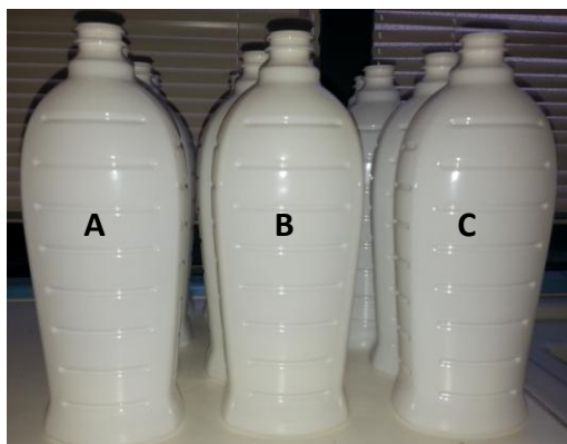
Figure 2. White 1 liter bottle for seeds oils (DANTE design). A) 31g 100% V-PET bottle; B) 31g 50% R-PET/V-PET bottle; C) 31g 100% R-PET bottles.
