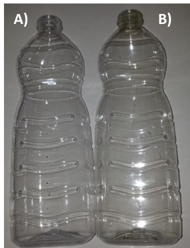
Figure 1. Clear 1 liter bottle for seeds oils (COOP design). A) 31g 100% V-PET bottle; B) 31g 50% R-PET/V-PET bottle.
