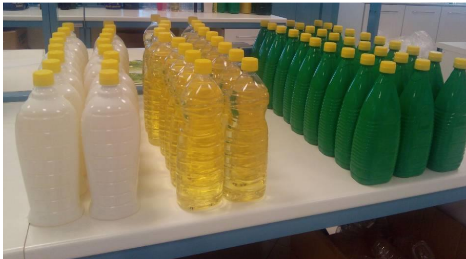
Photo 4. PCR-PET and PET bottles filled with sunflower oil stored on a shelf for 180 days at room temperature (23±5°C) in diffuse lighting condition for the shelf-life test.
