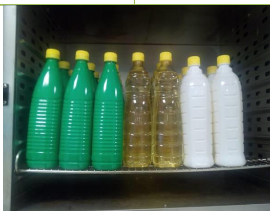
Photo 1. PCR-PET and PET bottles filled with sunflower oil stored in a climatic chamber for 90 days at 40°C for the accelerated shelf-life test.
